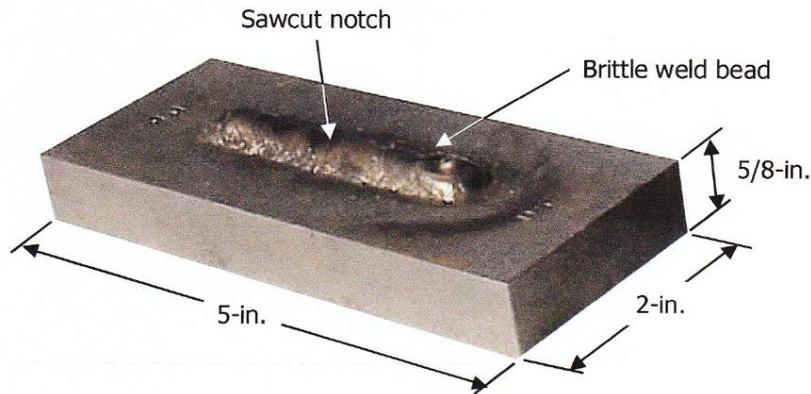
Drop Weight specimen (ASTM E 208)
