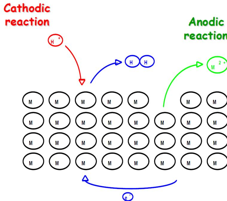
Aqueous corrosion (corrosion in LWRs)
