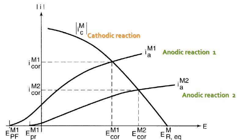
If the cathodic reaction rate is constant, free corrosion potential decreases when corrosion rate increase
