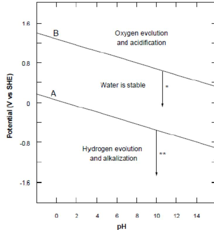
Figure 1.3 Thermodynamic stability of water, oxygen, and hydrogen. (A is the equilibrium line for the reaction:  $H_2 = 2H^+ + 2e^-$ . B is the equilibrium line for the reaction:  $2H_2O = O_2 + 4H^+ + 4e^-$ . \* indicates increasing thermodynamic driving force for cathodic oxygen reduction, as the potential falls below line B. \*\* indicates increasing thermodynamic driving force for cathodic hydrogen evolution, as the potential falls below line A.)
