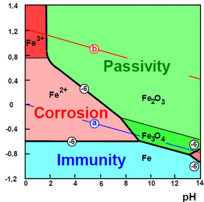
b) Corrosion diagram
