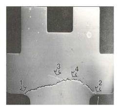
Metallographic examination of a cracked bolt
