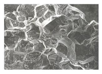
Intergranular fracture surface of a cracked bolt
