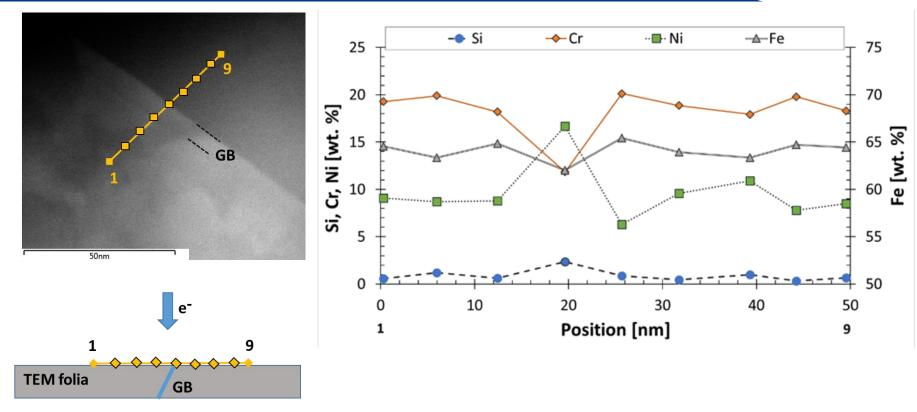
STEM EDS line scan across grain boundary; dashed line marks the position of grain boundary (GB) in the graph.
