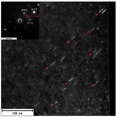
Frank loops marked by red arrows; the applied diffraction is shown in the small left corner frame.
