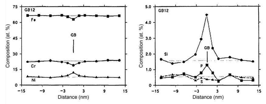
Conventional (V-shaped) grain boundary RIS profiles for a commercial purity 304 stainless steel neutron irradiated at 288 8C to 1.7 dpa [34]. Note depletion of iron and chromium at the boundary and enrichment of nickel, silicon and phosphorus[6]
