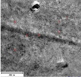
Cavities marking by red arrows: a) under-focused image, b) overfocused image Distribution of the size of the cavities dependence on the temperature
