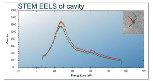
STEM EELS of cavity showing the scan line (black line) across the cavity where the EELS analysis was
