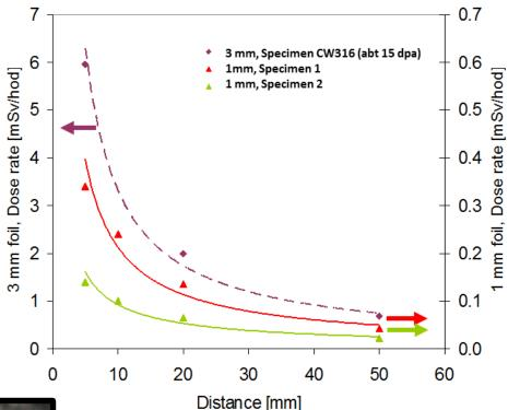
Figure: Dose rate from classical [3 mm] and currently developed [1 mm] TEM foils
