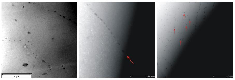
Ti-based precipitates distribution (right), decorating grain boundary of marked by red arrow (middle) and inside the austenitic grain (right), image taken in STEM mode using HAADF detector
