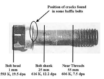
Examples are shown in (a) and (b) of the small cavities (encircled) present in a low density in the 1-mm bolt head position.
