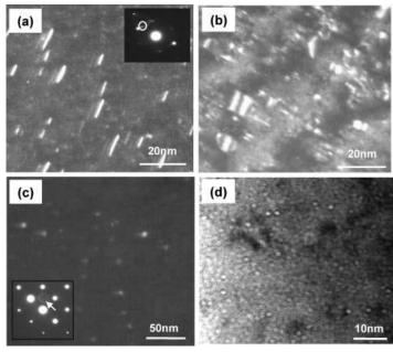
TEM images showing microstructural features observed in CW type 316 SSs PWR-irradiated to 53 dpa: (a) rel-rod dark field image of dislocation loops; (b) dark field image of dislocation loops and black dots; (c) dark field image of Ni3Si precipitates; and (d) defocused image of bubbles [Fukuya K, Fujii K, Nishioka M, Kitsunai Y. Evolution of microstructure and microchemistry in cold-worked 316 stainless steels under PWR irradiation. J Nucl Sci Technol. 2006;43:159–173.].
