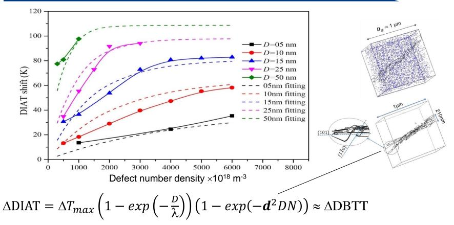
N: defect number density (in nm<sup>-3</sup>); D: defect size (in nm); **3 material-dependent scaling parameters** ( $\Delta T_{max}$ , d and  $\lambda$ )
