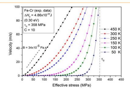
$$v_{screw}(\tau^*, T) = \frac{8\pi b(\tau^*)^2}{\mu Bh} X' \exp\left(-\frac{\Delta G(\tau^*, T)}{k_B T}\right)$$
