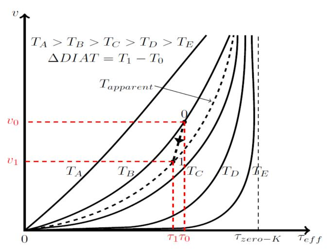
$T_{apparent} - T_0$  = Defect-Induced Apparent straining Temperature shift ( $\Delta$ DIAT)
