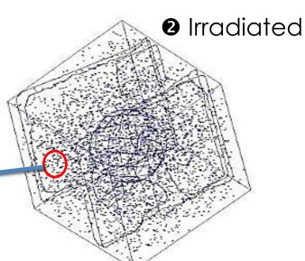
$T_{irr}$ =400°C, dose = 1 dpa, defect size D = 50 nm
