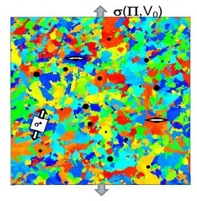
Example grain field with stress mapping
