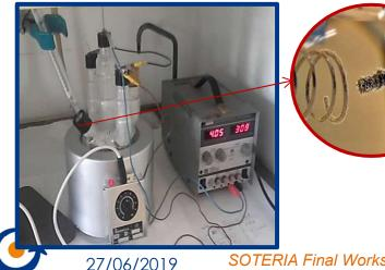
After cathodic hydrogen charging  $\epsilon$  martensite and  $\alpha$ ' martensite phases are detected by GIXRD
